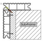
If Installing SwitchBoard with an overhang (max 25mm), It may be necessary to screw at an increased angle into the sub-frame.
