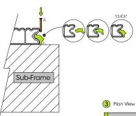
Butt the next board up to the clips and secure this board as shown in step 3. Repeat for all remaining boards.
