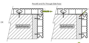
If installing SwitchBoard with an overhang (max 25mm), it may be necessary to screw at an increased angle into the sub-frame.
