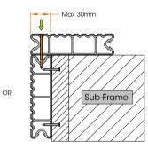
If installing SwitchBoard with an overhang (max 25mm), it may be necessary to screw at an angle into the sub-frame. The screw head must be within 30mm of the deck board edge to ensure trim coverage.
